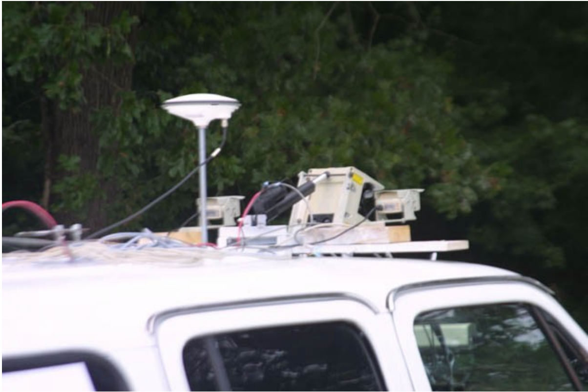
Downward Looking SICK Lidar, Stereo Cameras & GPS Unit
